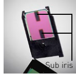
The sub iris cuts light leakage.
